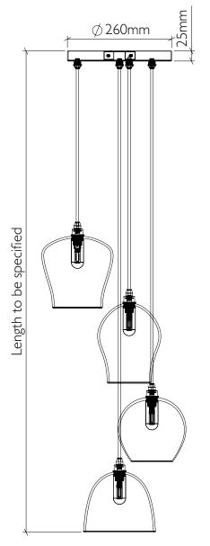
Product code IP65\_4CHD Materials Hand-blown glass, metal fittings Fitting IP65 with G9 LED bulb Flex Single braid fabric finished flex Length to be specified (non-adjustable)
